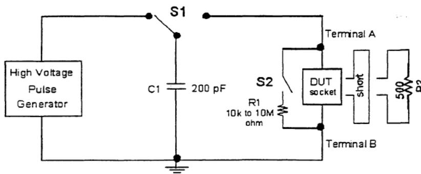
Figure 1 — Typical equivalent MM ESD circuit
