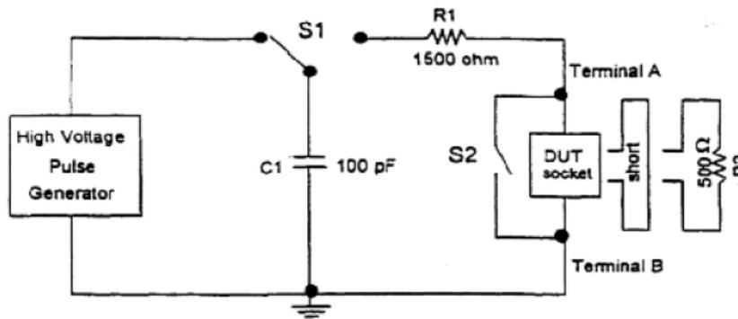
Figure 1 — Typical equivalent HBM ESD circuit
